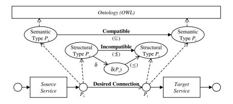
Fig. 5. A semantically valid, but structurally invalid connection.
