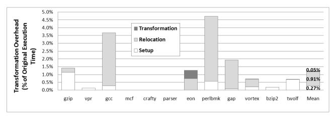
Fig. 4. Application overhead caused by preparing the code for instrumentation but without any instrumentation inserted.
