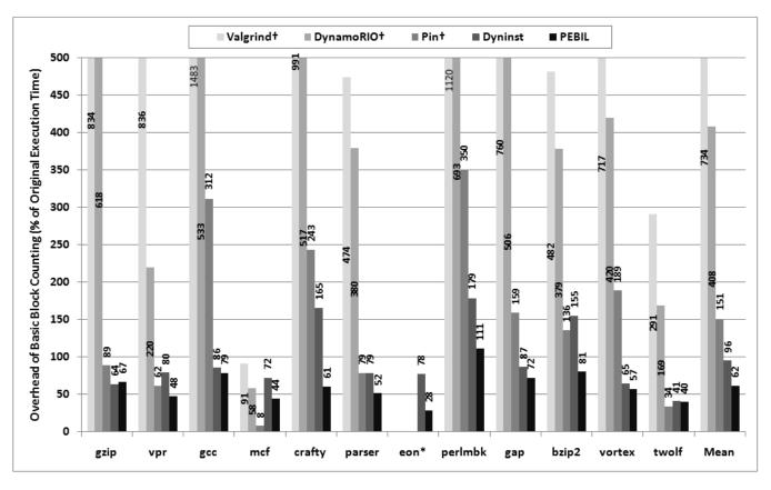
Fig. 5. Performance of several x86 instrumentation tools with basic block counting instrumentation.
