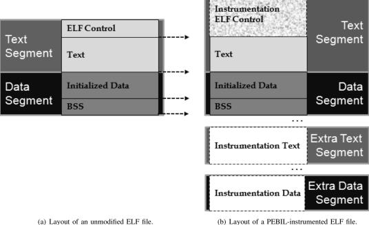
Fig. 1. (a) and (b) show that the text required by an instrumentation tool is prepended to the application text and the data required by an instrumentation tool is appended to the data application data.
